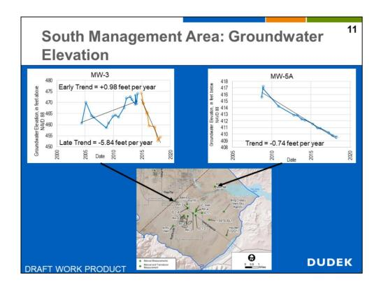
Well MW-5A located in the Borrego Sink in the SMA indicates a declining groundwater trend of 0.74 feet per year since 2008 when the well was drilled and completed. This well is located far from large pumping centers and likely provides.
